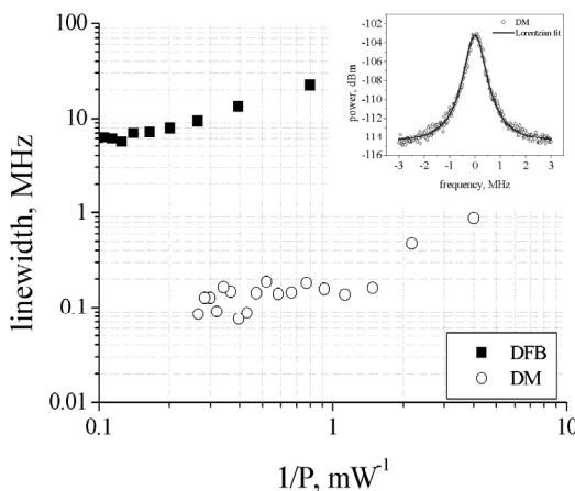
**Fig. 3.** Comparison DFB and DMLD sources using the measured variation of emission linewidth Vs inverse power,  $1/P$ . Inset: A typical self-heterodyne spectrum with a Lorentzian fit taken at a bias current of 40mA.
