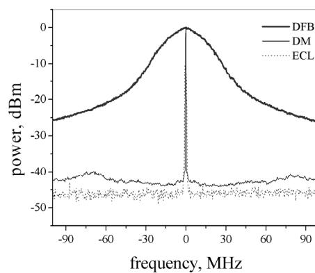
**Fig. 2.** Measured delayed self-heterodyne spectra where the offset modulation frequency (880 MHz) has been subtracted. Three spectra are shown (i) a DFB LD, (ii) a DMLD and (iii) an ECL
